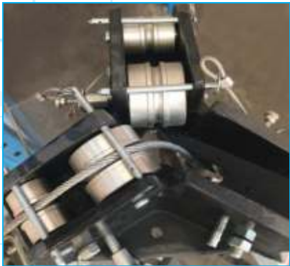
This Tripod is a Double Pulley Tripod design for usage of Winch of 6.0 mm wire rope.
